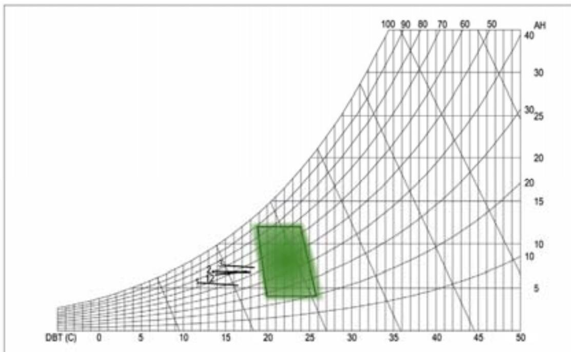
The second diagram illustrates the comfort zone for the mid seasons. The chart shows that temperatures below 21°C with a corresponding relative humidity of about 30% to 100% or temperatures above 28°C with a corresponding relative humidity of about 30% to 90% are not comfortable.
